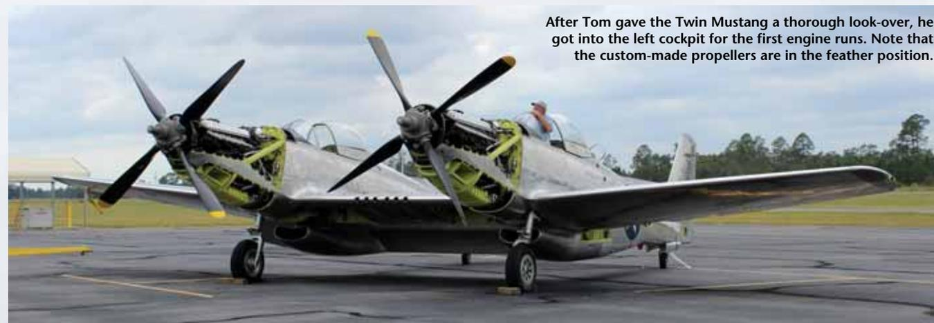
After Tom gave the Twin Mustang a thorough look-over, he got into the left cockpit for the first engine runs. Note that the custom-made propellers are in the feather position.
